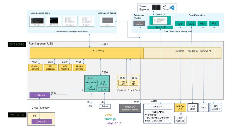
The diagram shows the default port numbers that are used by Zowe. These are dependent on each instance of Zowe and are held in the Zowe YAML configuration file.
