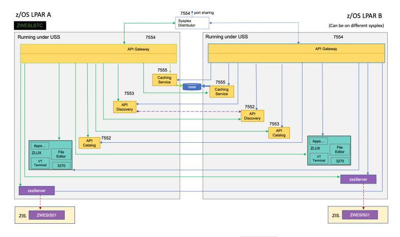
Zowe has high availability feature build-in. To enable this feature, you can define haInstances section in your YAML configuration file.
